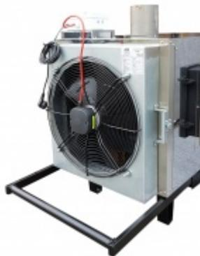
In addition, hot air is distributed using an axial fan.
