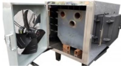
The heat needed to heat the object is obtained by means of thermal exchange between the exhaust fumes and clean air, via a heat exchanger.
